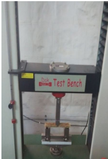
Fig.6 Flexural Test on Composite Material
