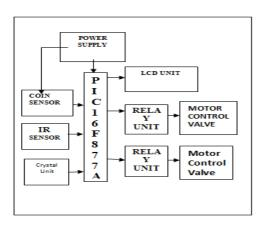
Figure 1.0 block diagram of Water Wending Machine
