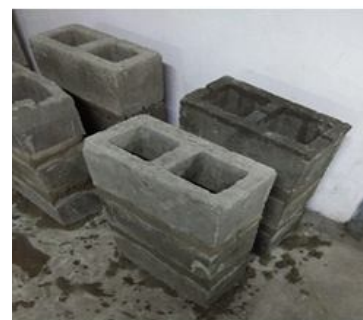
Fig. 7 Prism of hollow concrete block
