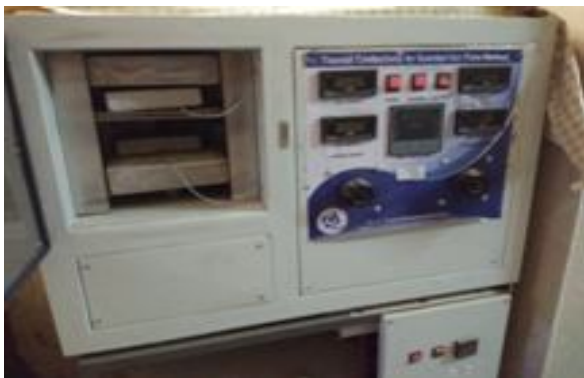
Fig. 8 guarded hot plate for measuring the thermal conductivity
