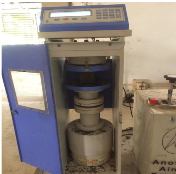
Figure 2: Compressive Strength Machine Setup
