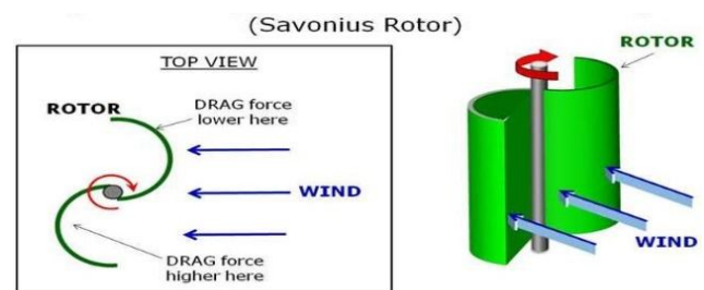
Fig 1 : Savonius blade design
