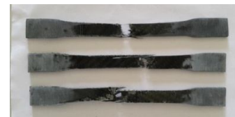
Figure 5.2 Test specimen after tensile test
