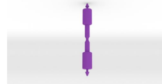
Figure 5.1 Tensile test of the specimen.
