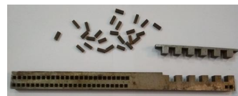
Figure 4.1 Square cut in a flat plate of M6 HSS.
