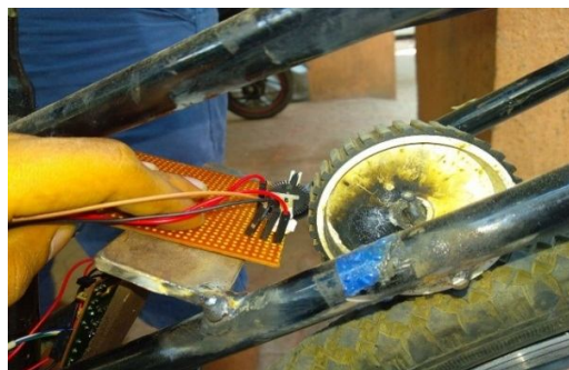
Fig - 3 Y-axis wheel connected to the caster wheel
