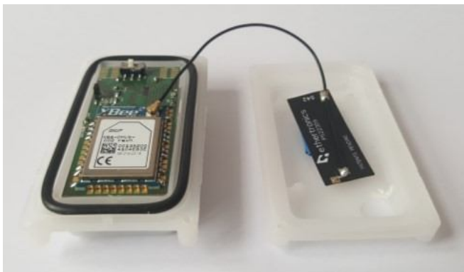
Fig. 2. Smart ZigBee tags placed in waterproof package
