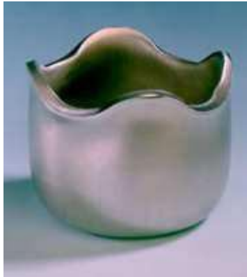
Fig. Earing in deep drawing
