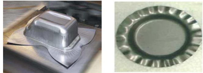
Fig: Example of Wrinkling
