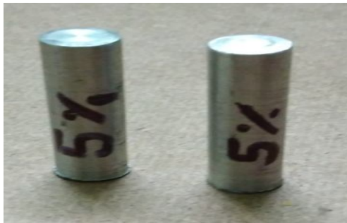
Figure1 (a)Specimens for wear test
