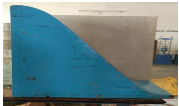
Figure 2.1: Ogee spillway physical model by wood
