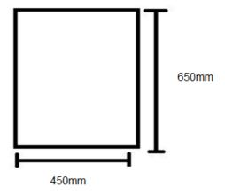
Frame design for safety FOR 25\*25\*3 L angle mild steel channel
