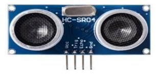
An ultrasonic sensor is a device that can measure the distance to an object by using sound waves. It measures distance by sending out a sound wave at a specific frequency and listening for that sound wave to bounce back. By recording the elapsed time between the sound wave being generated and the sound wave bouncing back, it is possible to calculate the distance between the sonar sensor and the object.
