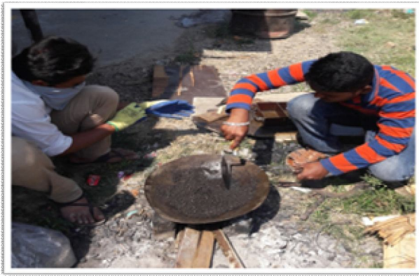
Step 1: Sand heating with flame
