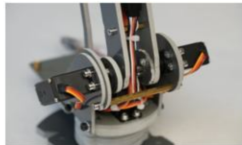
Fig.2 Three servo meters attached next to base
