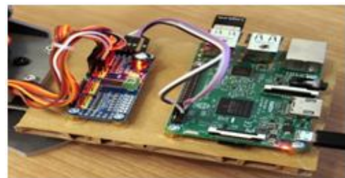
Fig. 6 Raspberry Pi connected with a PCA9685 Servo controller
