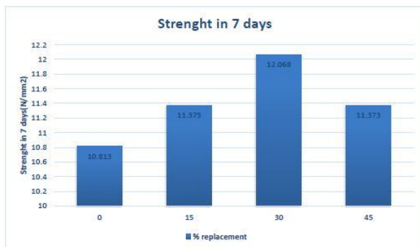
Fig 3.1 7 th day compressive strength
