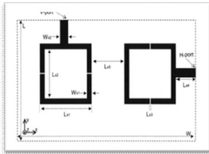
The layout of the S-band antenna, where  $L = 106$ ,  $W=183$ ,  $Ls1 = 53.89$ ,  $Ls2 = 44.6$ ,  $Ls3 = 0.94$ ,  $Ls4 = 19.31$ ,  $Ls5=34.17$ ,  $Ws1=4.9$ , and  $Ws2 = 7.8$  (all dimensions are in mm).
