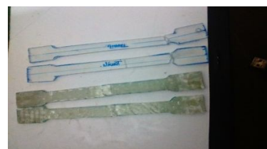
Figure 5.2 Test specimen for tensile test
