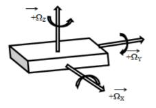
Gyro sensor is an angular rate sensor or angular velocity sensors. In simple terms, angular velocity is the change in rotational angle per unit of time. The accelerometer measures the acceleration +g (gravitational acceleration). Its function is based on elasticity of very small semiconductor beam inside the IC. Deflection of this beam is measured piezoelectricity. Gyro measures speed of angular rotation about an axis
