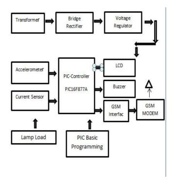
For protection against hazardous condition such as over current there is current sensor in model which will precisely detect the over current.
