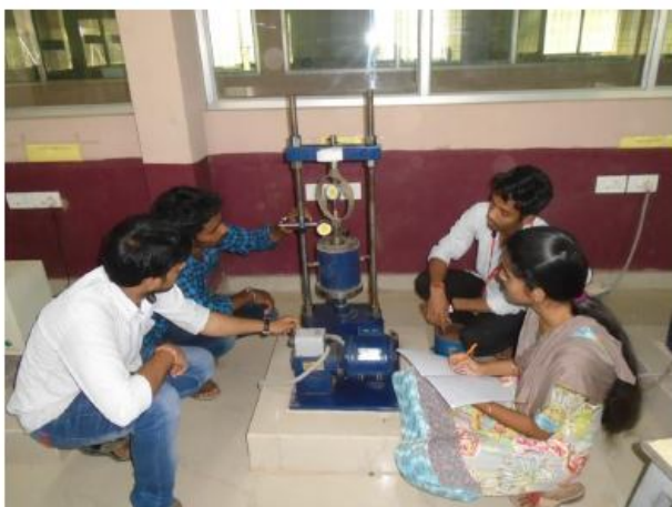
Fig 3.5 conducting CBR test
