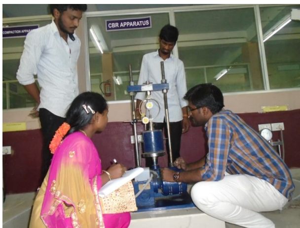
Fig Shows Conducting CBR test
