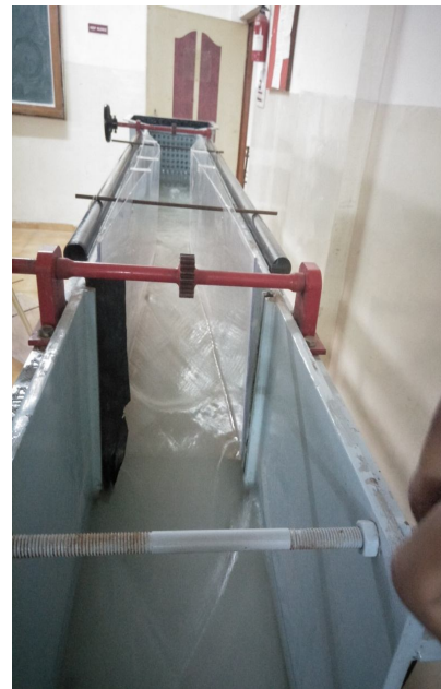
PIC 1: TRADITIONAL VENTURIFULME IN FLOATING CONDITION
