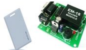
Figure 7.2 RFID Tag and Reader
