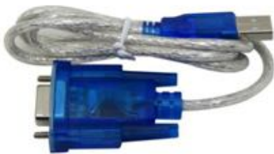
Fig 6: USB to RS232 convertor
