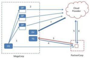
This architecture consists of three main components, they are a data processor (DP), that processes data before it is sent to the cloud; a data verifier (DV), that checks whether the data in the cloud has been tampered with; and a token generator (TG), that generates tokens that enable the cloud storage provider to retrieve segments of customer data; and a credential generator that implements an access control policy by issuing credentials to the various parties in the system
