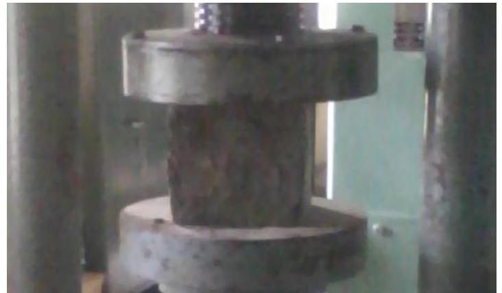
Fig 4.2 Compressive test of concrete cube
