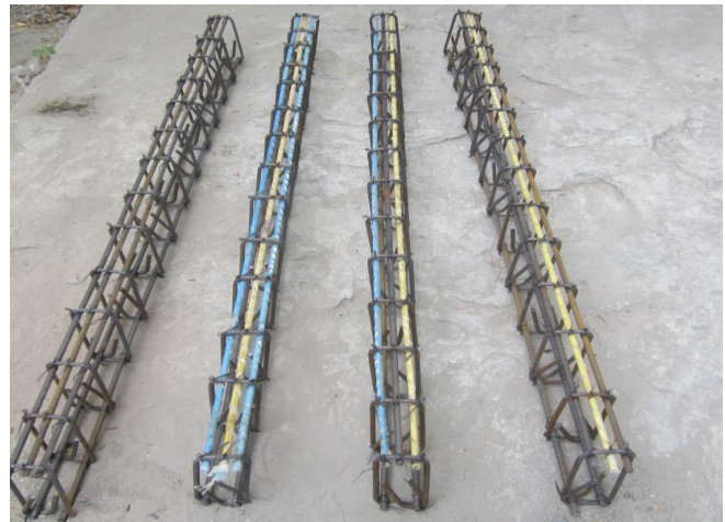
Figure 3.1 Reinforcing details for the tested beam
