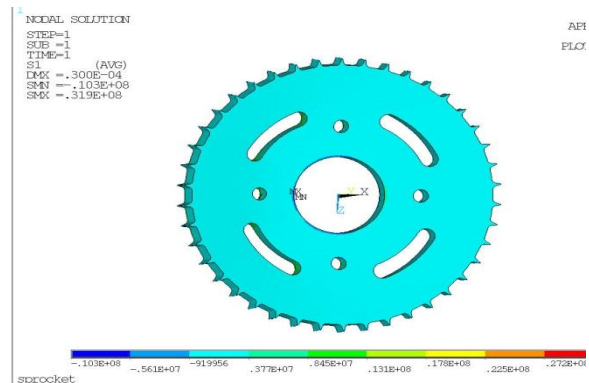
Figure11. The 1 st principal stress developed
