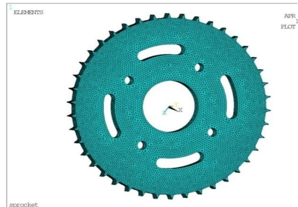
Figure3. The meshed model is shown in the above figure.
