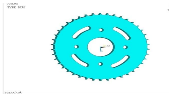
Figure2. 3D model in the Ansys environment
