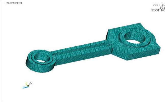
Figure.4. shows the Mesh model of connecting rod used for analysis.
