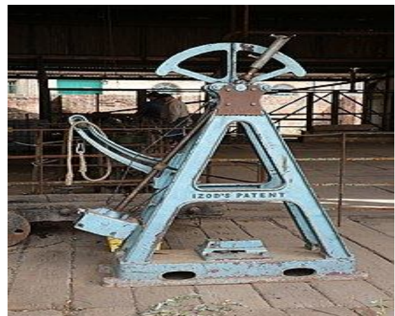
Figure 5 : Izod Impact testing machine
