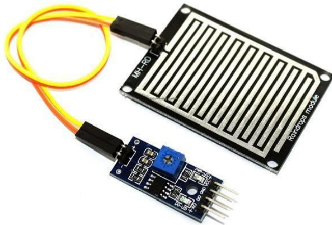
Fig 4. Prototype for Rain detector sensor
