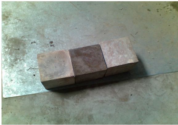
Figure 2. Cement Concrete Cubes
