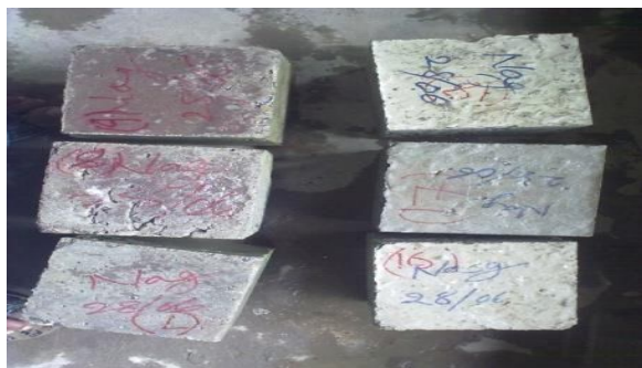
Figure 9. Concrete cubes after immersion in MgSO 4
