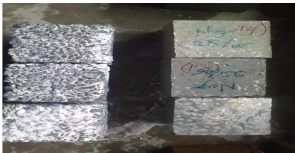
Figure 8. Concrete cubes after acid immersion in H 2 SO 4
