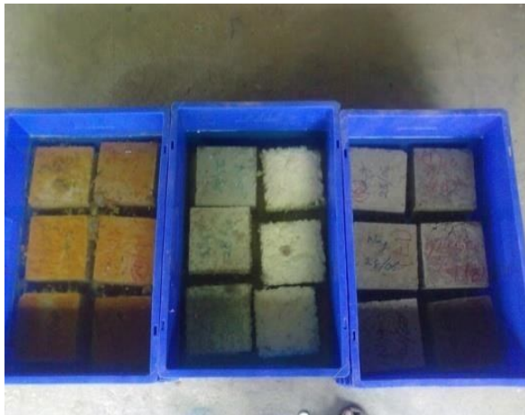
Figure 6. Immersion of concrete cubes
