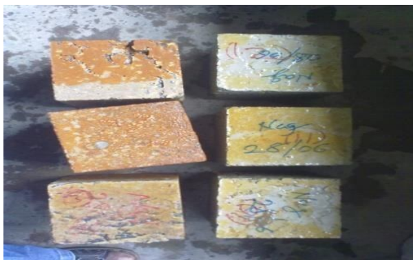
Figure 7. chemical solutions (HCl, H 2 SO 4 and MgSO 4 )
