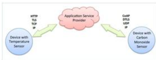
Fig 3: Device – to – Cloud Communications
