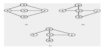
The routes ABCE and ABE, have both link AB and node B in common. It doesn't have a disjoint path. The routes ABE, ACE, and ADE have no common node or link.
