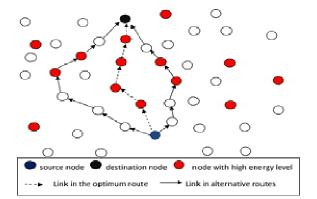
The FF-AOMDV broadcast the RREQ in order to collect the information regarding the available routes towards the destination as it is shown in the above figure. Here fitness function performs the scan on the network in order to locate the nodes that have the higher level of energy.
