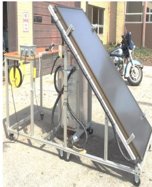
Figure 1. Solar water heater set up
