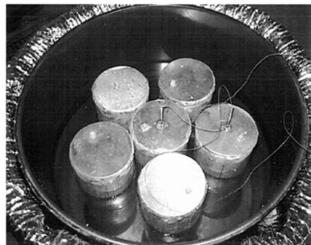
Figure 4. Heat Exchangers inside the Water Reservoir
