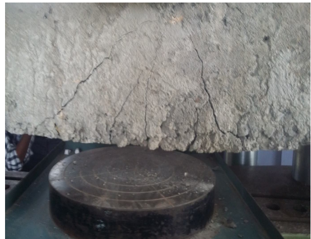
Figure 4.3 Failure pattern in conventional beam
