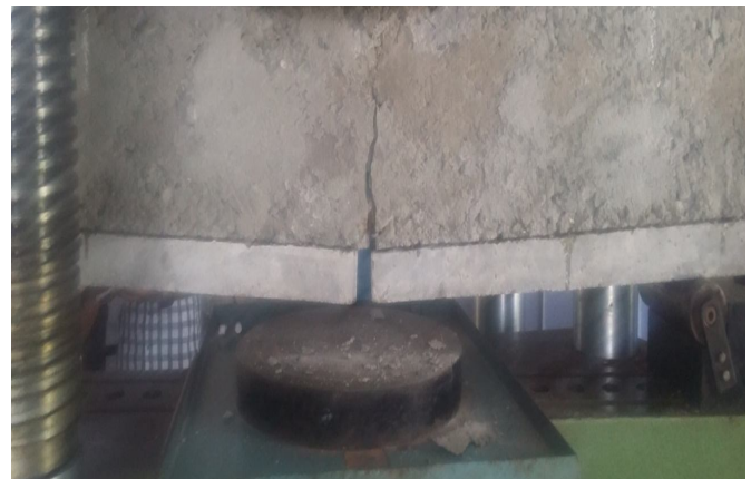
Figure 4.4 Failure pattern in strengthened RC beam
