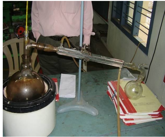
Figure1. Experimental setup of fractional distillation to extract plasti diesel (PD) from liquid hydro carbons
