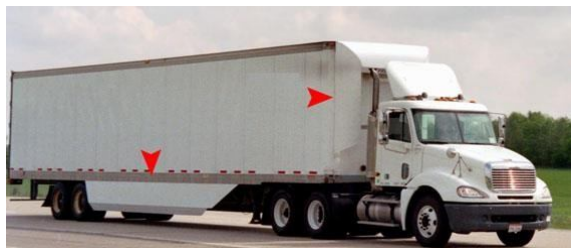
Fig1.1 A truck with added bodywork ontop of thecab to reduce drag.
