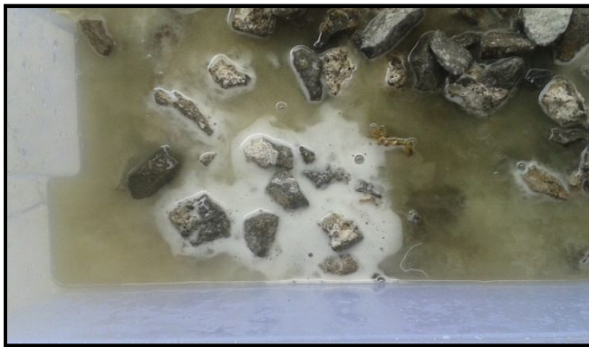
Figure 2. Acid treatment of RCA
