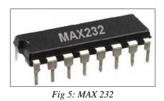
In this project MAX232 which is a dual driver/receiver IC that includes a capacitive voltage generator in which supplies sufficient voltage to the zigbee connected to it. Each pin in the IC will delivers an output voltage of 5 volts. Each driver converts inputs levels into various EIA-232 levels. The P3\_0 (RX) and P3\_1 (TX) pin of controller is connected to the max 232 driver and the TX and RX pin of max 232 is connected to the GSM modem or PC.
