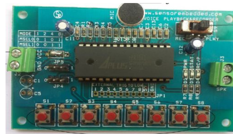
Fig.11 APR33a3 Voice Playback Processor
