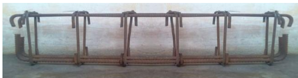
Reinforcement of OSB
