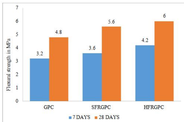
Fig. 5.4 Variation of Flexural Strength at 7th and 28th day
