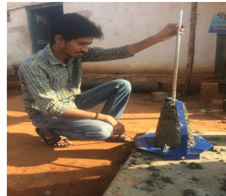
. Slump cone test
