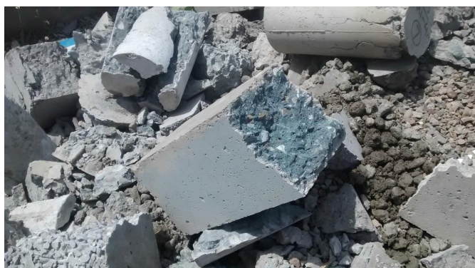
Figure 1. Failure sample of geo polymer concrete
