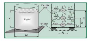
The parameters of the tank: H is the liquid height, R is the radius and  $t_h$  is the average thickness of the tank wall. The lumped masses are expressed in terms of the liquid mass (m) and it is taken from Haroun's model.
