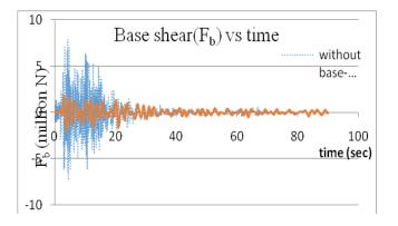
Similarly it can be observed the impulsive displacement decreases with time period of Base-isolation system. Moreover, for a relatively short isolation period (say less than 2.2 s) the base shear reduces rapidly and after that it become nearly flat for Tb > 2.5 sec
