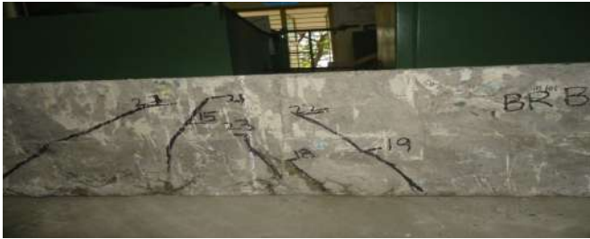
Figure 14. Appearance of BRB after test
