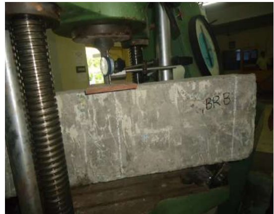
Figure 13. Appearance of BRB before test
