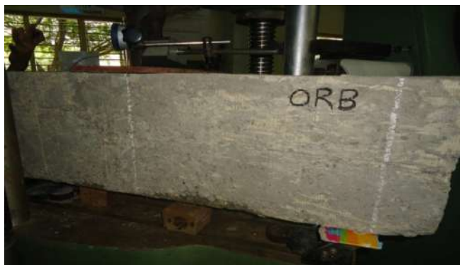
Figure 16. Appearance of ORB before test
