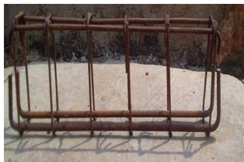
Figure 9. Reinforcement of URB
