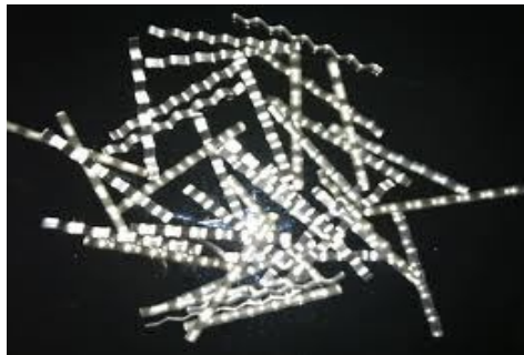
Figure 1: Crimped steel fiber
