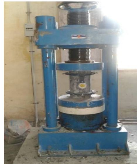
Fig.6 test setup of e- for concrete
