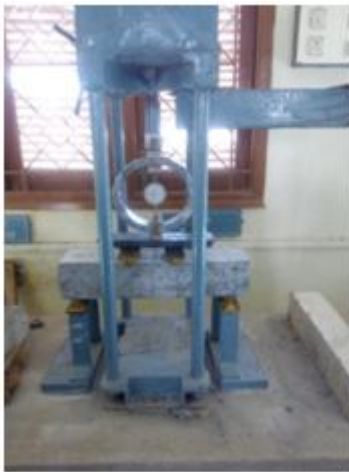
Fig. 4 Flexural Strength Testing Machine
