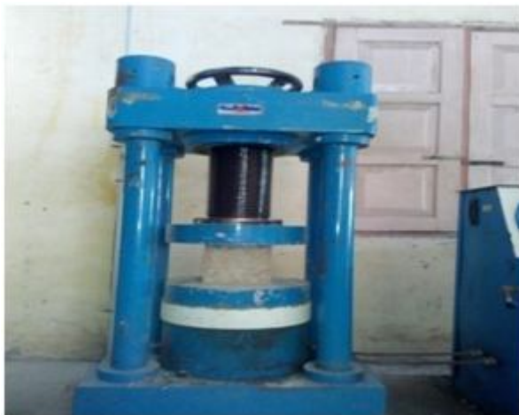
Fig. 2 Compressive Strength Testing Machine
